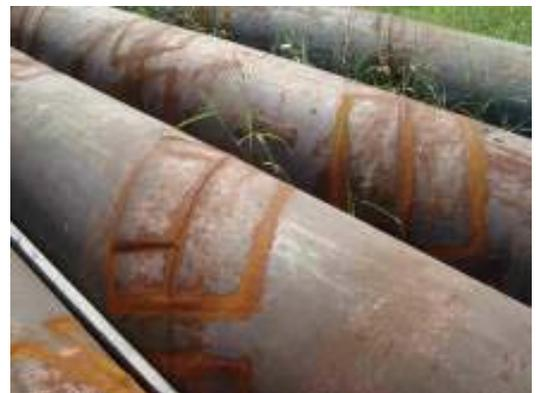
Figure 7. Test Spools containing manufactured spiral weld defects.
