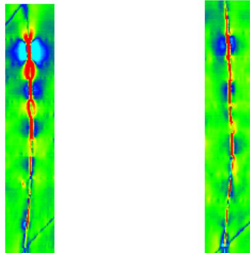
Figure 13. Plots of MFL data for various girth weld anomalies of interest
