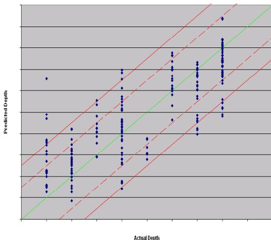
Figure 12. Initial Sizing Performance of Spiral Weld Anomaly Model.
