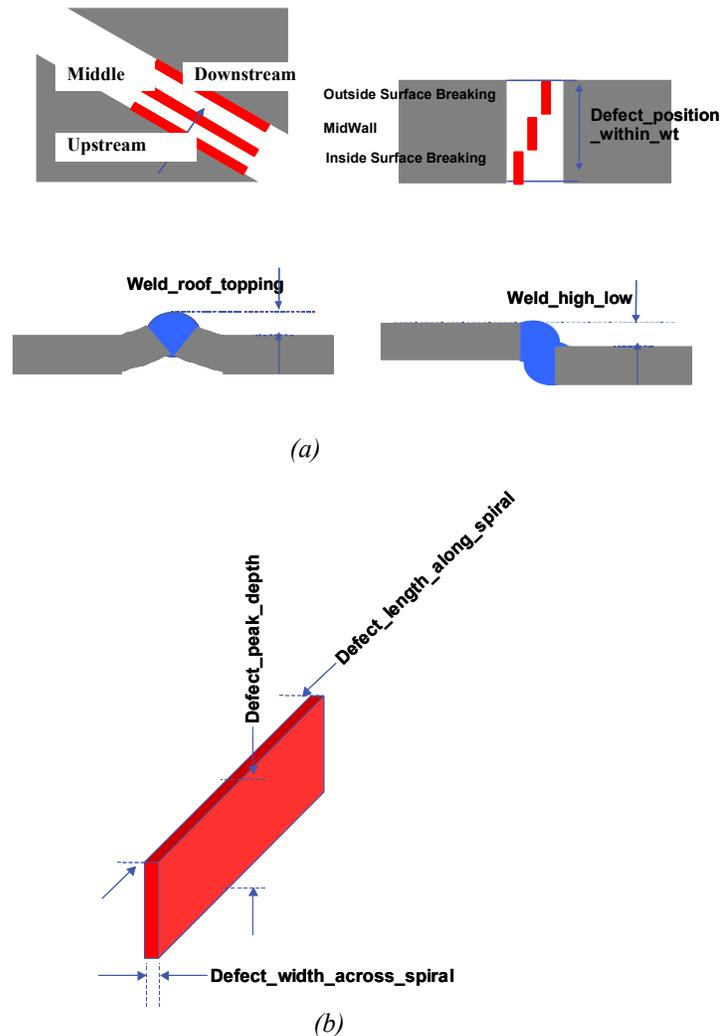
Figure 6. Spiral weld feature parameter definitions (a) Defect Location, b) Defect Dimensions
