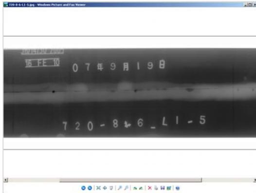
Figure 5 Radiographic Image - Example of Lack of Fusion spiral weld defect
