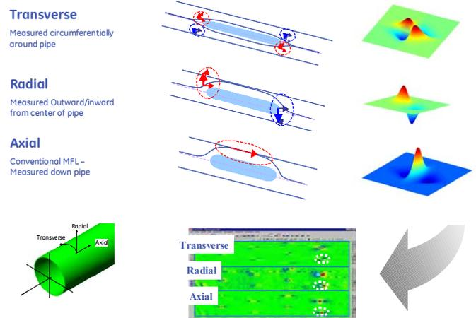
Figure. 1 Overview of Signal Responses from multi-axis sensor MFL inspection
