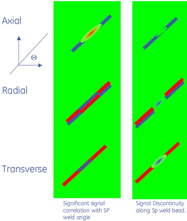
Figure. 8 Spirally aligned features of interest
